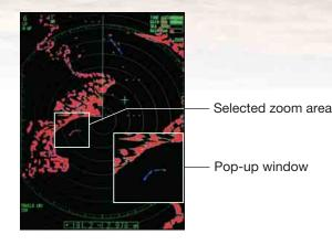
With the optional ARP board ARP-11, up to 10 targets can be acquired and tracked on the radar screen. Additionally, up to 100 AIS targets can be presented with appropriate AIS data input.
