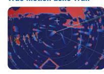
When connected with a heading sensor and position receiver, i.e. GPS, the FR-8002 series can display True Echo Trails to present true target movements in accordance with their speed-over-ground and course-over-ground. This mode provides intuitive monitoring of moving targets.
