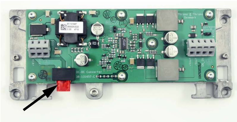
Figure 3: Replacing the fuse in the Power Converter
