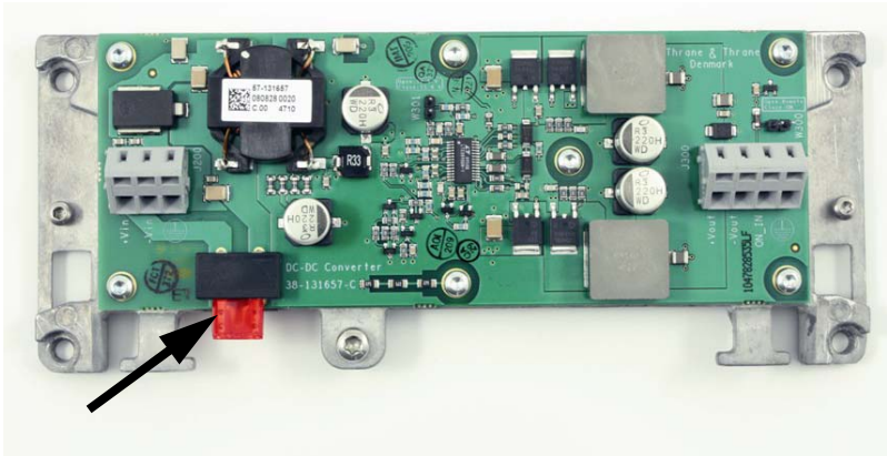
Figure 4: Replacing the fuse in the Power Converter
